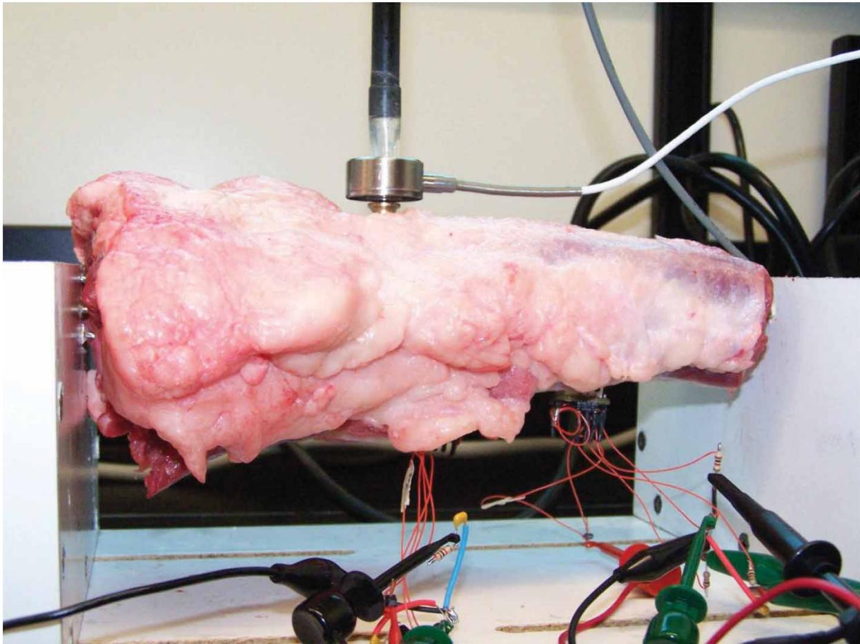
FIGURE 2. Imparted mechanics set-up. 100 lb load cell is attached to cleaned section of central vertebrae [five in total] and aligned with stylus of device. Three-dimensional accelerometer on central vertebrae [bottom] measures stylus effects on *in situ* vertebrae.
